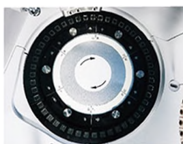
Reaction Tray 37±0.2°C, real-time monitor.
