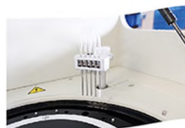
Washing Probe Independent 5-step washing system.
