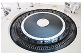
Reaction Tray 37±0.2°C, real-time monitor.
