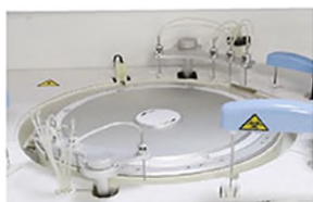
Reaction Tray 37±0.1°C, water bath
