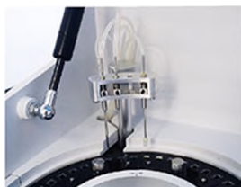
Washing Probe Independent 3 -step washing system.
