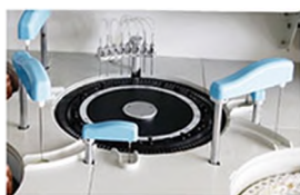
Reaction Tray 37±0.1°C, real-time monitor.
