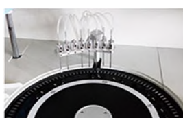
Washing Probe Independent 7-step washing system.
