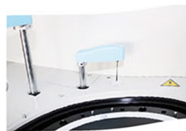
Mixer Probe Teflon coating to avoid cross contamination.
