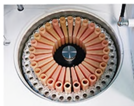
Reagent Tray Refrigerated tray with independent switch.
