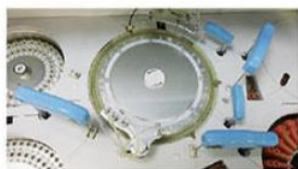
Reaction Tray 37±0.1°C, water bath
