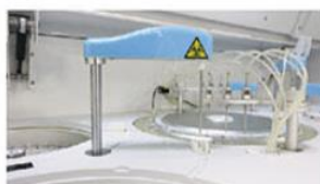
Sample Probe Liquid level sensor function Anti collision function Reagent volume real-time detection
