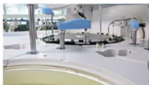
Mixer Probe Dual mixer, auto frequency adjustment
