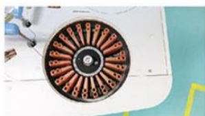
Reagent Tray 2~8°C cooling for 24 hours
