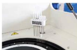
Washing Probe Independent 4-step washing system.
