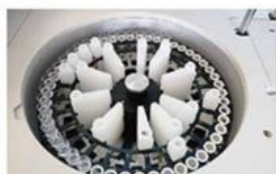
Reagent Tray 2~8°C cooling for 24 hours.
