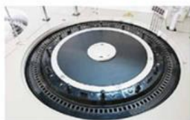
Reaction Tray 37±0.1°C, real-time monitor.
